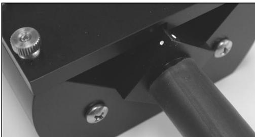
For best repeatability it is important to insert collectors in a consistent orientation. To facilitate this, collectors may have a pair of white dots marked on them. These dots should always be facing up, that is, toward the flat top plate, as shown in Figure 5.
