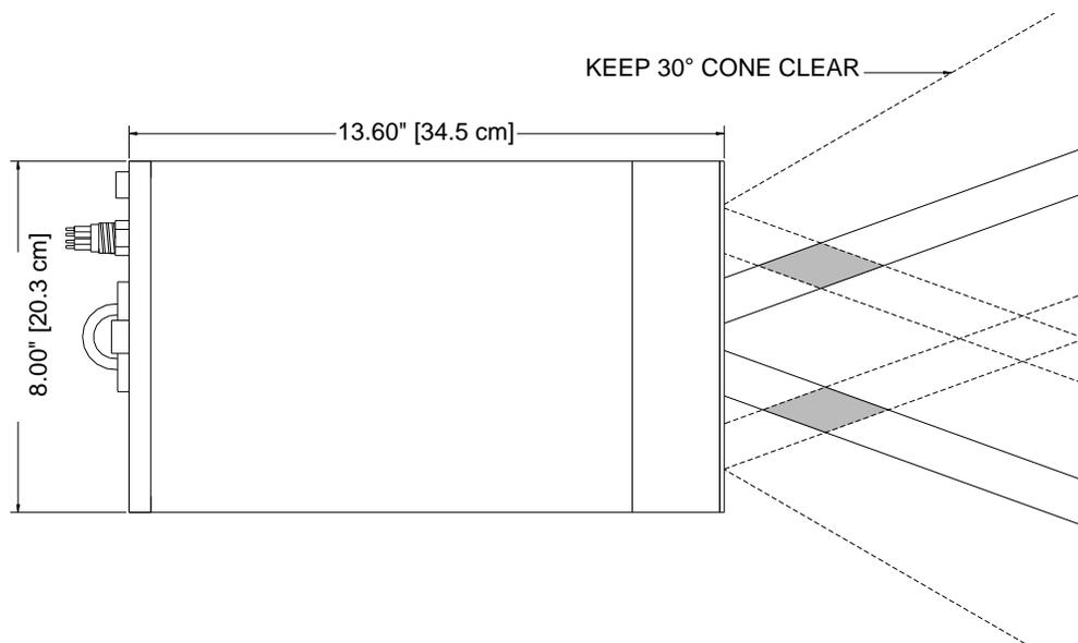
**Figure 4: HydroScat-6 side view without cage**
