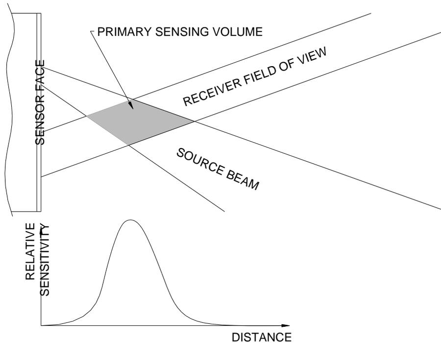
**Figure 1: Side View of Backscattering Measurement Geometry**
